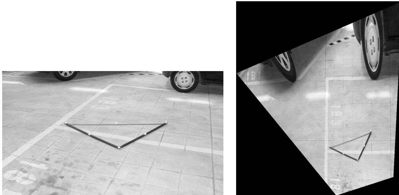
Fig. 12. A perspective image and a ortho-rectified image of the floor plane
