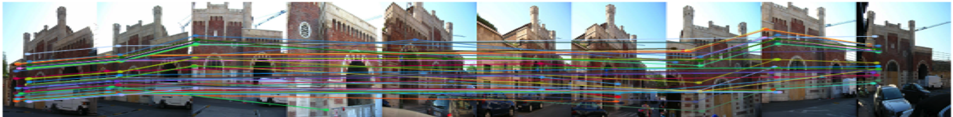
Fig. 7. Keypoints are connected into multiple-view correspondences, called tracks .
