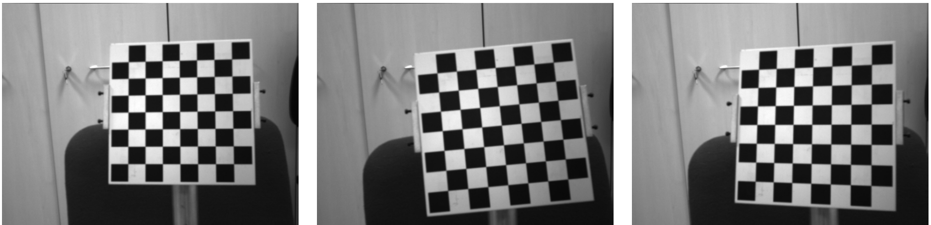
Fig. 21. Images of a planar calibration pattern. The points used for calibration are the corners of the black squares.
