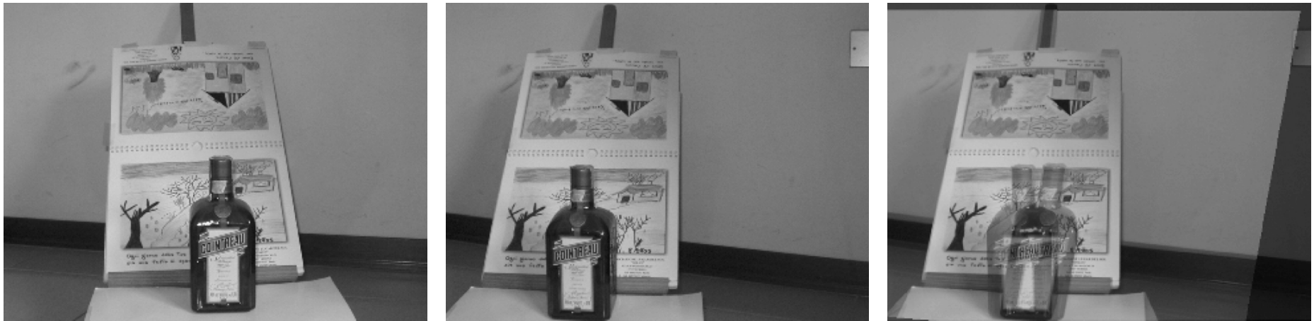
Fig. 9. Left and right images. The leftmost image is a superposition of the warped left image and the right image. The reference plane exactly coincide. However, points off the plane (such as the bottle) do not coincide.
