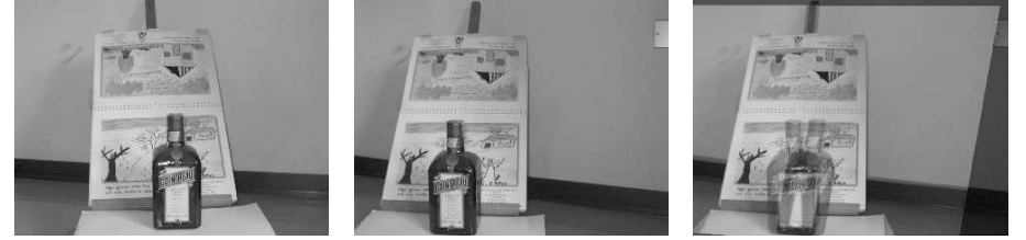
Fig. 8. Left and right images. The leftmost image is a superposition of the warped left image and the right image. The reference plane exactly coincides. However, points off the plane (such as the bottle) do not coincide.
