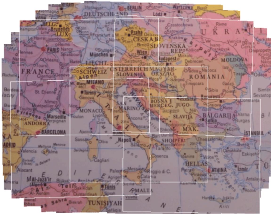
Fig. 10. Planar mosaic with components location shown as white outlines.
