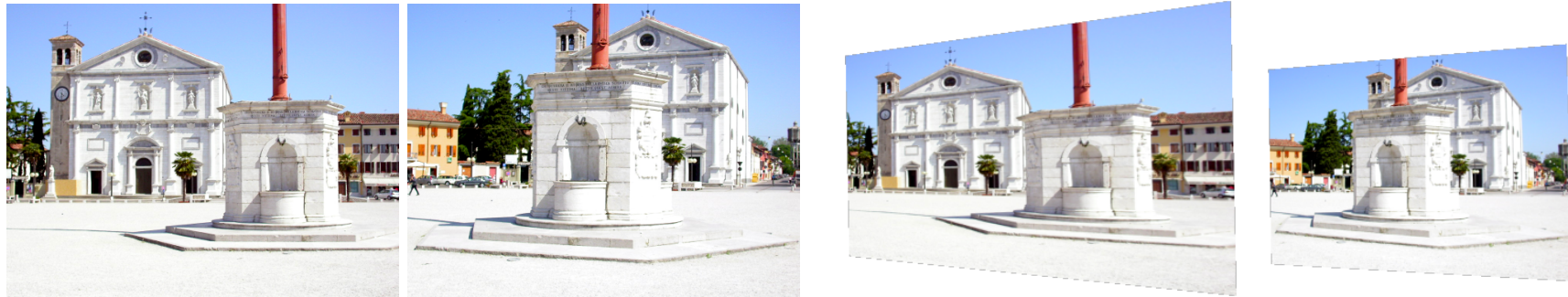
Fig. 21. Original and rectified stereo pair.
