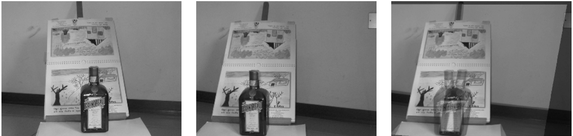
Fig. 9. Left and right images. The leftmost image is a superposition of the warped left image and the right image. The reference plane exactly coincide. However, points off the plane (such as the bottle) do not coincide.
