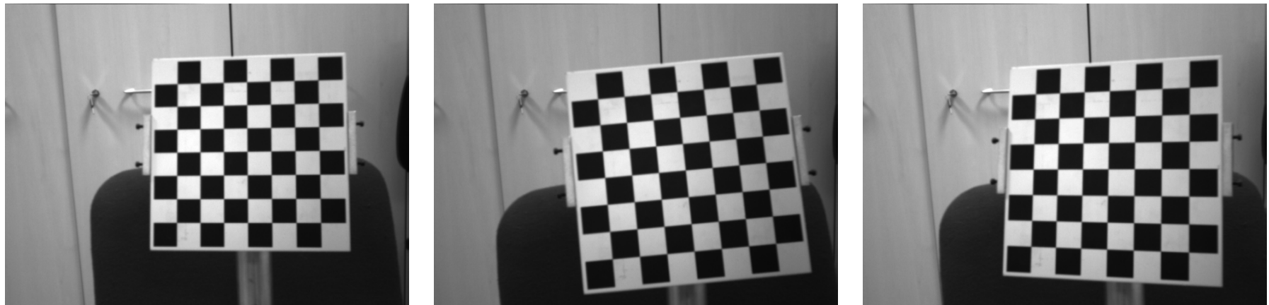
Fig. 19. Images of a planar calibration pattern. The points used for calibration are the corners of the black squares.
