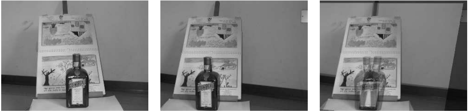
Fig. 15. Left and right images. The leftmost image is a superposition of the warped left image and the right image. The reference plane exactly coincide. However, points off the plane (such as the bottle) do not coincide.
