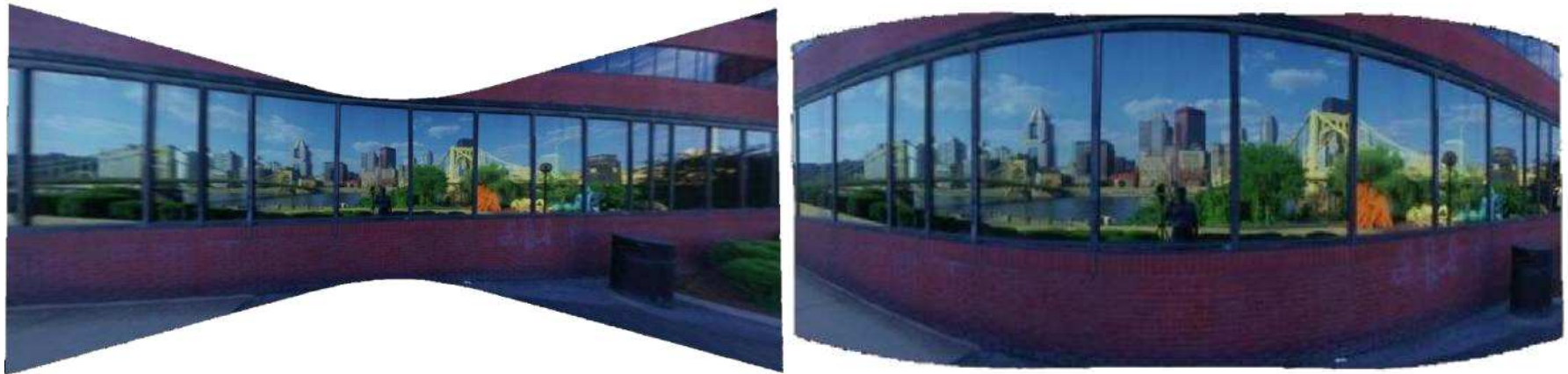
Fig. 18. Planar panoramic mosaic (right) and its projection onto a cylinder (left).
