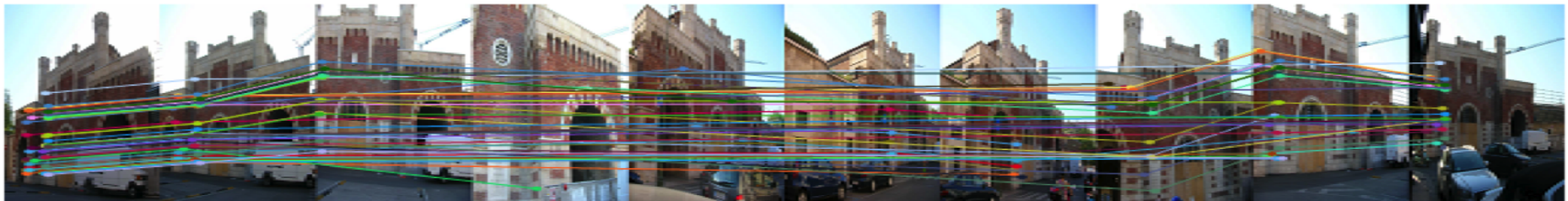
Fig. 5: Keypoints are connected into multiple-view correspondences, called tracks .
