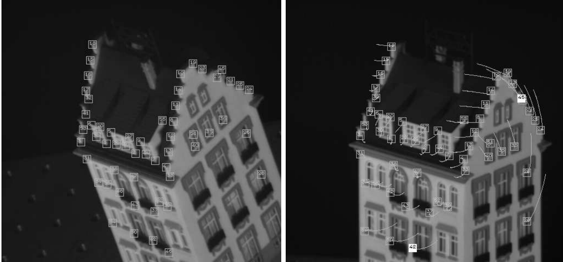
Figure 45: First (left) and last frame of the “Hotel” sequence. In the last frame, filled windows indicate features rejected by the robust tracker.
