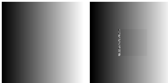
Figure 33: Gray-level ramp stereo pair. The central square has disparity 5 pixel, the background 2 pixel.
