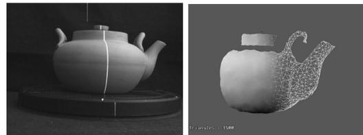
Figure 1: Left: laser stripe projected onto a teapot; Right: 3-D reconstruction of a single view of the teapot.
