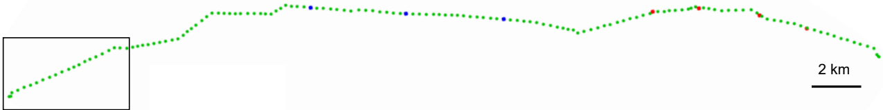
Figure 8. Visualization of results on the 36 km-long test line. Pylons correctly detected (green), false positives (red), and false negatives (blue). Reconstructed cables for the part of the power line in the black box are shown in Fig. 1.
