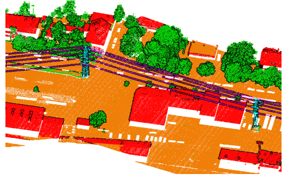
Figure 3. Example of the results obtained from the segmentation algorithm. Classes: ground (orange), vegetation (green), building (red), cable (pink), pylon (cyan).
