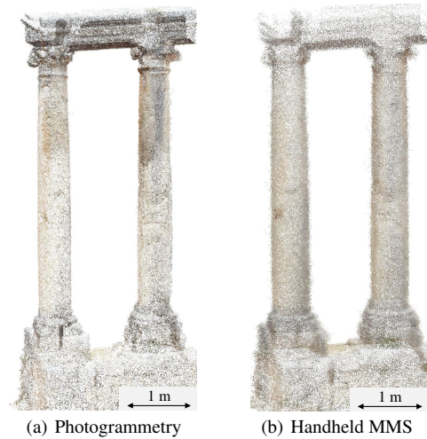
Figure 10. Detail of the point clouds, showing the columns of the temple. The higher noise that characterizes the handheld MMS can be appreciated in (b).
