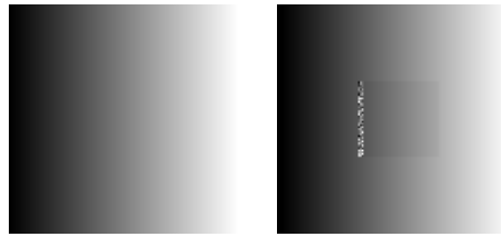
Figure 9. Stereo pair. The central square has disparity 5 pixel, the background 2 pixel.
