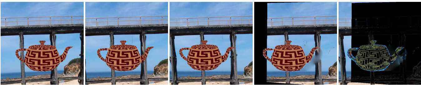
Fig. 1. The first three images from left to right have been generated with OpenGL. The fourth have been extrapolated from the first two with our algorithm. The last one is the difference between the extrapolated image and the ground-truth.
