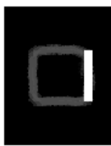
Fig. 5. Computed disparity map (left) by SMW for the square random-dot stereogram and its uncertainty (right). MAE is 0.019.
