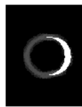
Fig. 6. Computed disparity map (left) by SMW for the circle random-dot stereogram and its uncertainty (right). MAE is 0.026.
