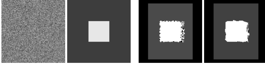
Fig. 3. Square random-dot stereogram. The left image of the stereogram is shown (left). The right one is computed by warping the latter with a given disparity pattern (right). The square has disparity 10 pixel, the background 3 pixel.
