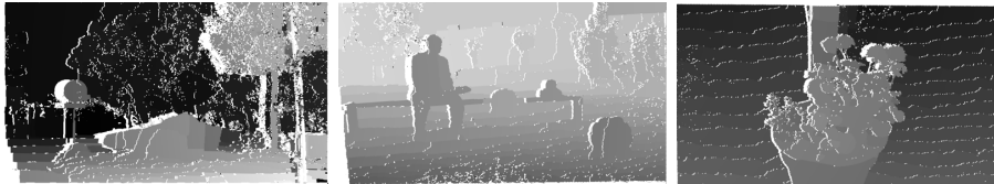
Fig. 2. Parallax maps obtained from the stereo matching.
