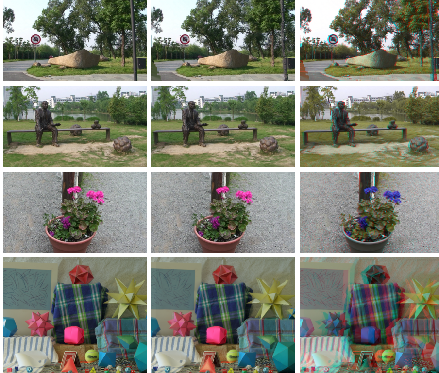
Fig. 3. Examples of the 3DS output. From left to right: reference image (left eye), virtual image (right eye), red-cyan anaglyph.
