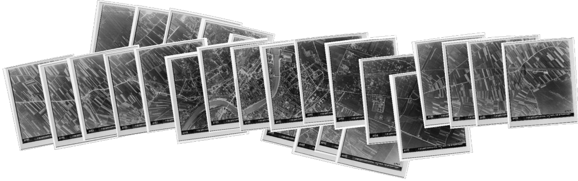
Fig. 1. An example of a sequence of exposures taken by the Royal Air Force (RAF) during WWII (from the AFN archive). The photos are placed in their relative positions by panoramic stitching, using [1].
