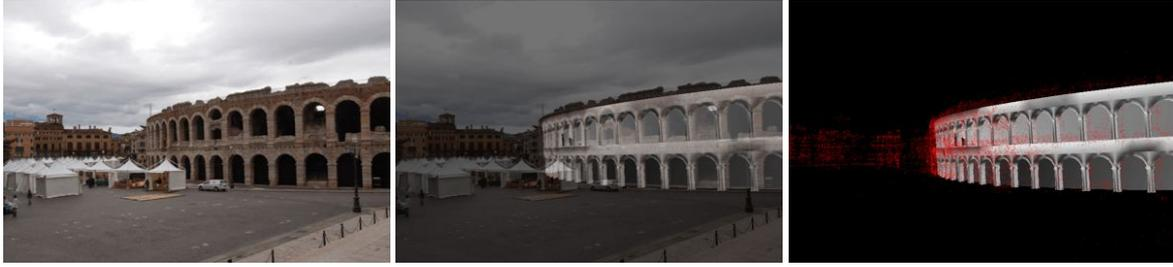
**Figure 4:** Example of mixed reality overlay from a localized view. On the left the original image; in the middle a superimposed 3D model of the Arena; on the right the 3D model with the points cloud in red.
