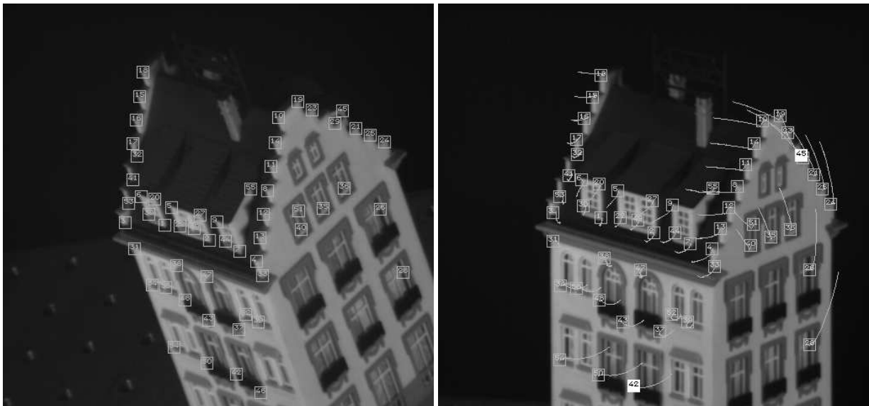
Fig. 2. First (left) and last frame of the Hotel sequence. In the last frame, filled windows indicate features rejected by the robust tracker.
