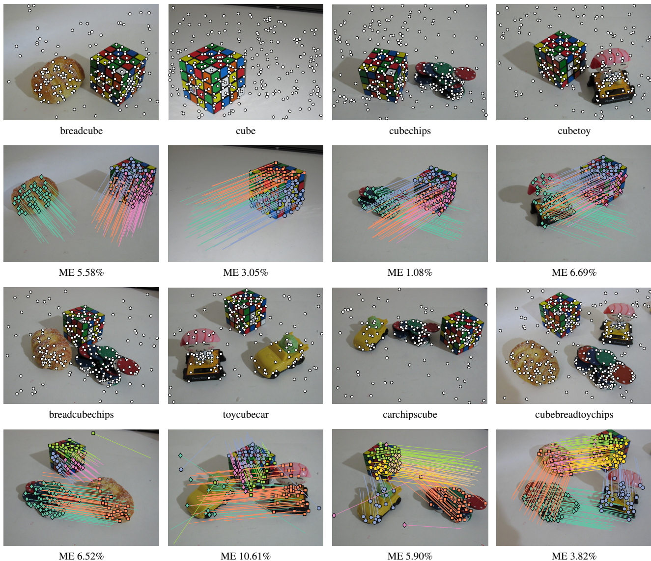
Figure 6: Homography and fundamental matrix fitting by MCT on cube* image pairs of the AdelaideRMF dataset. We sampled 5000 F matrices and 1000 H matrices per cluster. Odd rows: first input image with outlier-contaminated points overlaid. Even rows: F and H models superimposed on the second image (model assignment is colour coded).
