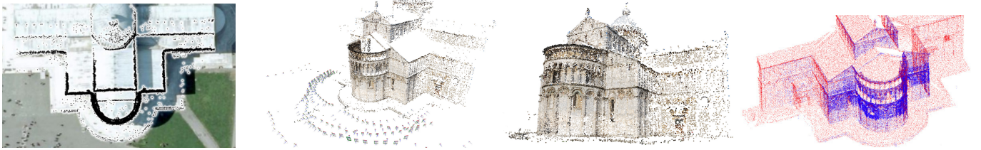
Figure 9: A top view and two perspective views of the reconstruction of “Duomo” (Pisa, Italy). In the last picture the point cloud (blue) is shown superimposed to the ground truth (red).
